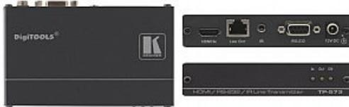
The TP-573 is a DGKat™ twisted pair transmitter for HDMI, bidirectional RS-232 and infrared signals. The TP-573 converts the input signals to a twisted pair signal and the TP-574 converts it back to HDMI, RS-232 and infrared signals
